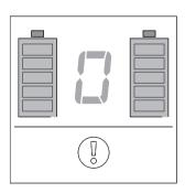
If an error is indicated according to the table on the following page and both battery symbols flash at the same time, the error indicated occurs in both wheels or in the battery packs of both wheels.
