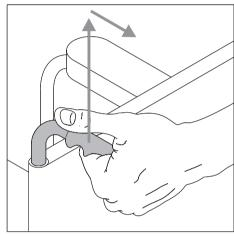
• At the same time, pull the wheelchair by its handles slightly to the top and rear until the wheelchair was raised and the anti-tippers engage in a fixed position.
