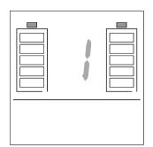
Push the button [23] on the remote control to simultaneously switch on both e-motion wheels in power stage 1.
