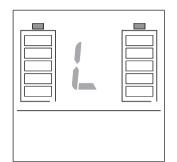
When activating the button lock, the following is shown in the display: the current charge status of the two battery packs, an "L" in alternating fashion, the power stage currently set (1 or 2) and in case an error occurs, the corresponding error code.
