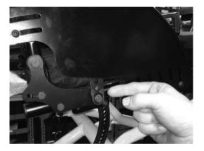
Click strap for Pro BB/Pro Tennis Series attached to seat or back frame using back bracket.
