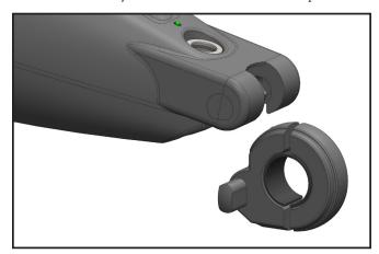
1. To attach the drive unit to the wheelchair, align the flats in the adaptive clamp with the receiving slots on the front, underside of the unit body [the drive unit will be angled slightly higher than horizontal]. Lower the receiving end of the drive unit over the extrusions of the clamp.
