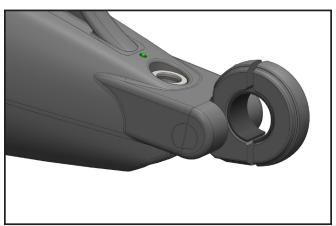
**2.** Rotate the unit downward to pivotally attach the drive unit to the clamp, and consequently the wheelchair.
