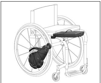
2. Lower the battery unit towards the seat of the wheel-chair. Position the upholstery of the seat between the bottom surface of the clip and the top surface of the battery housing. With the Button plug wire to the side, slide the unit back until the front surface of the upholstered seat is making contact with the handle.
